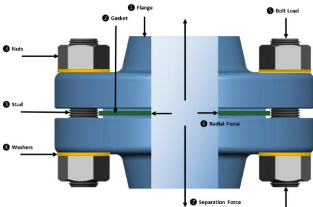
**1 Flange** Connects piping, valves, pumps and other related components together
