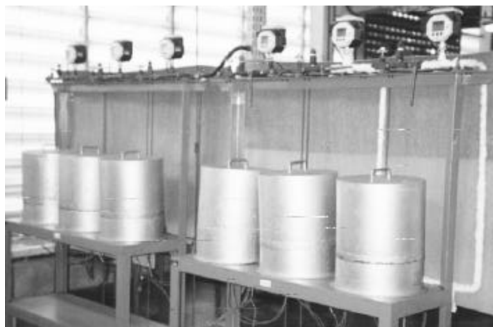
Fig.3: Class 150 and Class 300 test cells - insulated.
