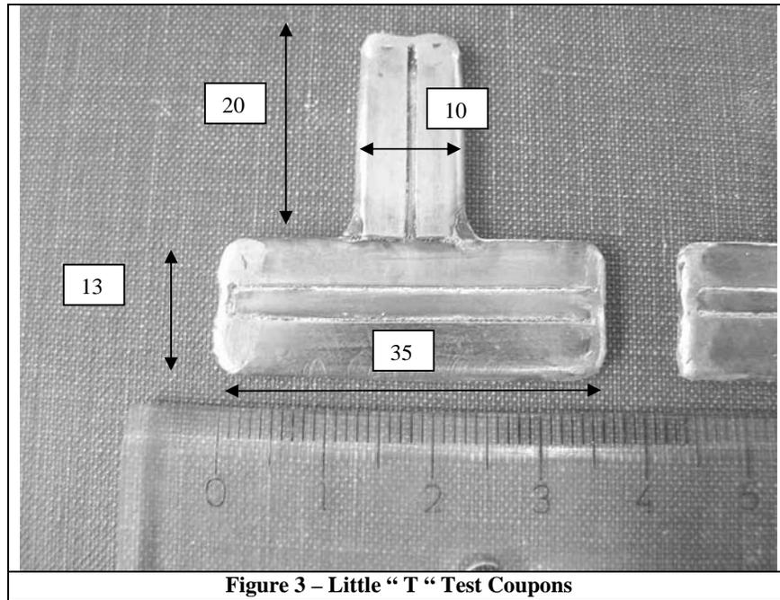
**Figure 3 – Little “T” Test Coupons**
