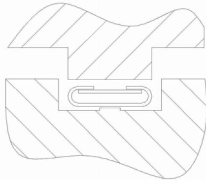
**Figure 17 – Flange with nubbin, gasket centered with groove. Overlap opposite nubbin.**
