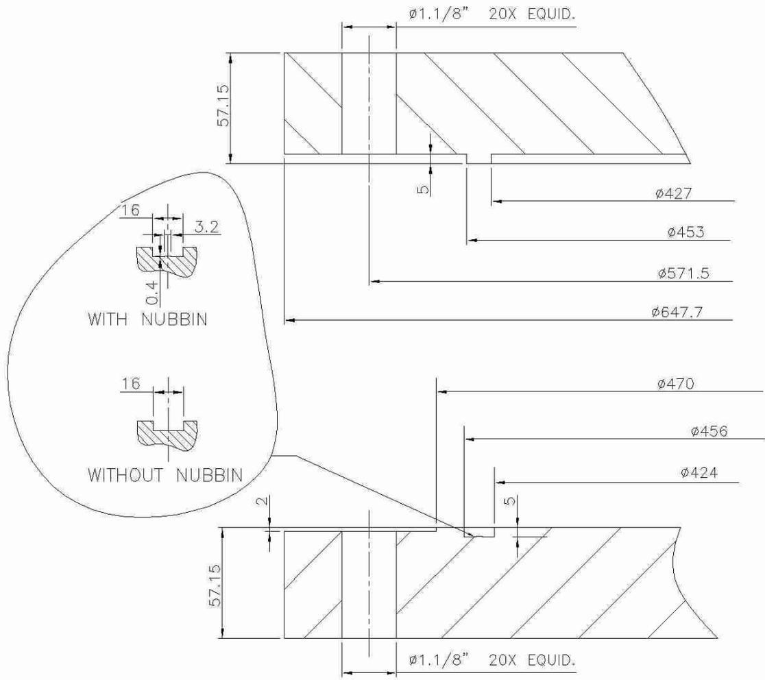
Figure 13 – Test flanges with nubbin and without nubbin.
