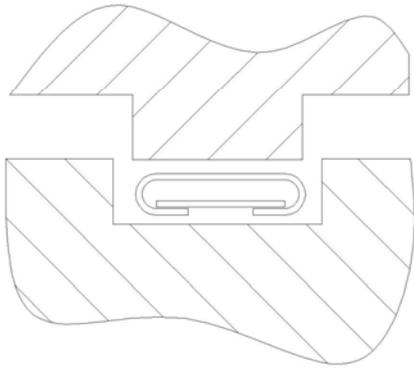
**Figure 14 – Flange without nubbin, gasket centered with groove. Overlap opposite male.**
