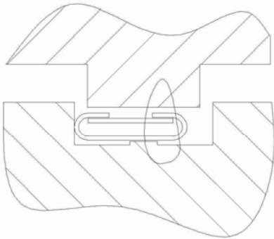
**Figure 16 – Flange with nubbin, gasket not centered with groove. Overlap opposite nubbin.**
