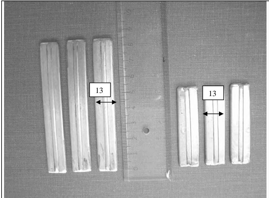
**Figure 1 – Straight Test Coupons without butt-welded joint**
