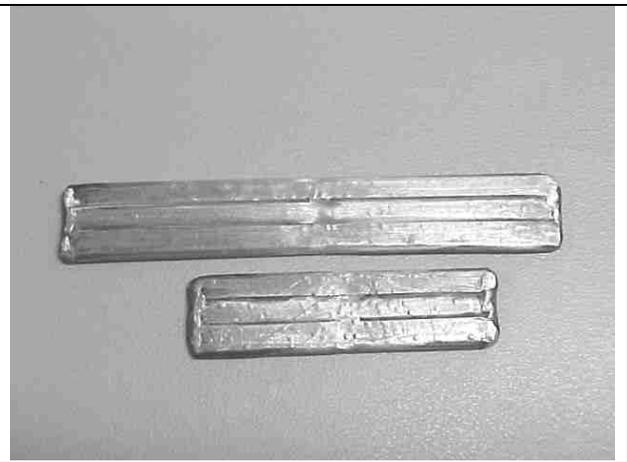
**Figure 5 – Straight test coupons with butt-welded joint**
