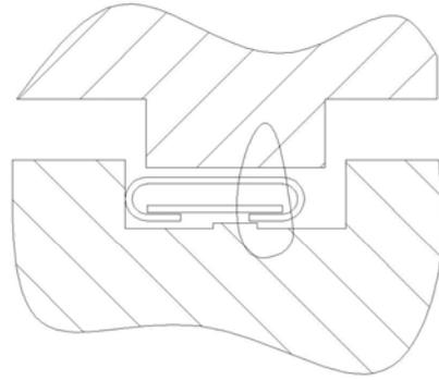
**Figure 15 – Flange with nubbin, gasket not centered with groove. Overlap opposite male.**
